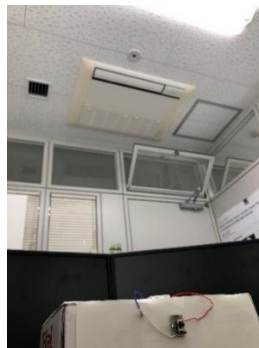
Fig. 8. OWPT at a 160 cm distance between the ceiling LED array and the optical receiver.
