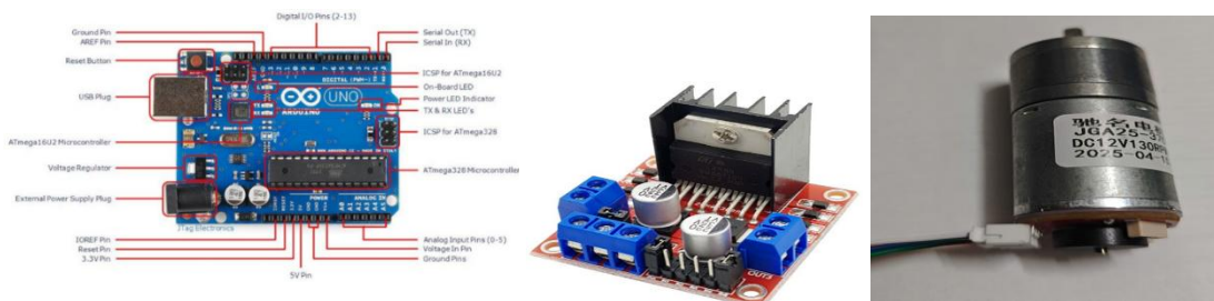
Figure 4. Control boards and encoder module
