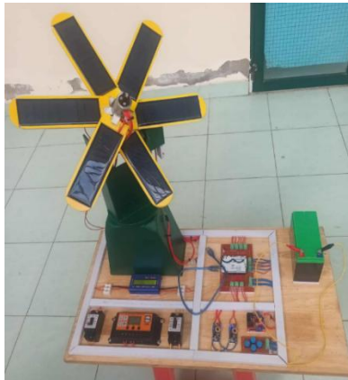
Fig. 4. The fabricated prototype of the sunflower inspired dual axis solar tracker
